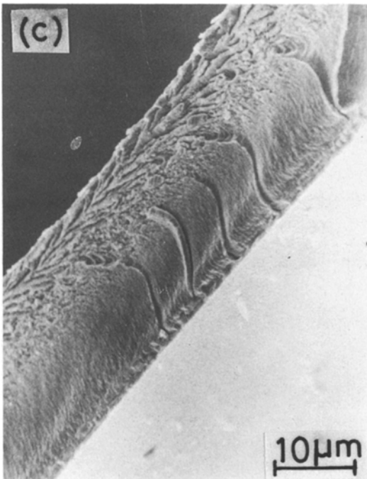
Figure 14 Fracture surfaces of the aged specimens in the second stage of heat treatment, where the ageing conditions are as follows; (a): aged at 623 K for 36 ksec, (b): aged at 723 K for 0.6 ksec, and (c): aged at 773 K for 0.6 ksec, respectively.
